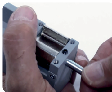
2.4 - Reinsert the pin and tighten the screw.
