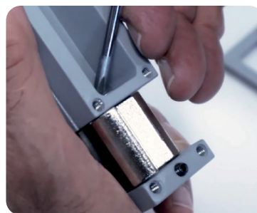
2.2 - Rotate the strike latch.
