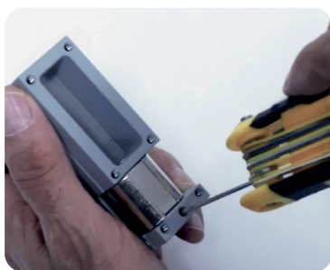
2.1 - Unscrew the security screw.
